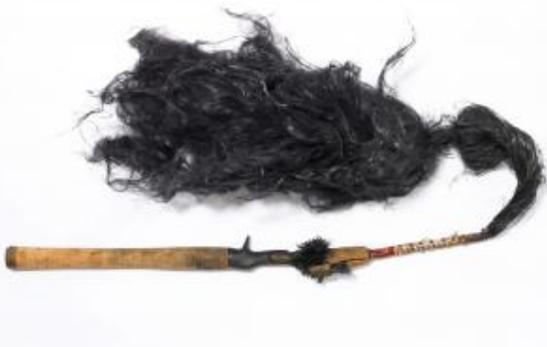
**This is the picture of a fly rod after a lightning strike.**
